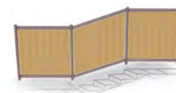
INCLINED ADAPTATION TO THE SLOPE
