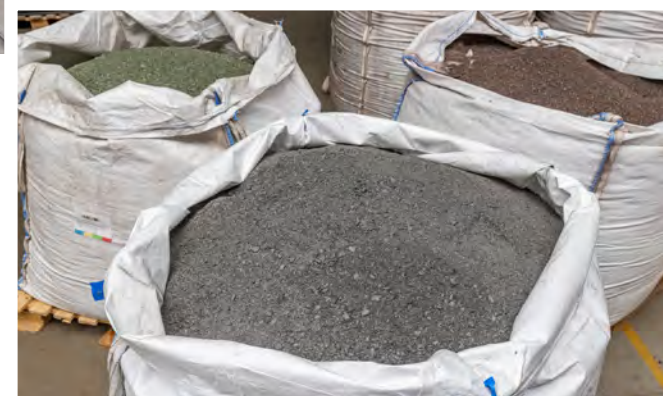
Worn-out decking boards that are returned to us from our take-back dealers are shredded – after separation by type – into a fine granulate. This is returned to the production cycle and used for the manufacture of new boards, which enables us to save valuable resources.
