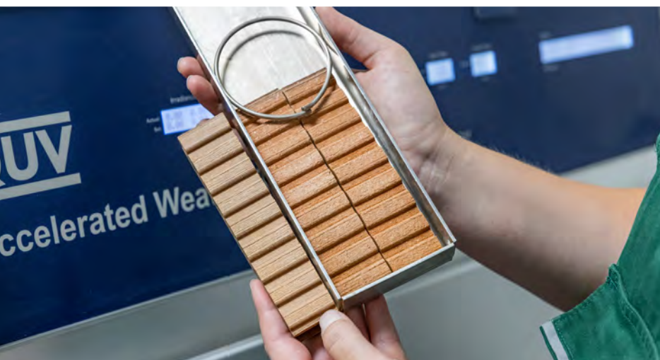
Left: A new megawood® board Right: the megawood® board that has been in the QUV tester since 2006
