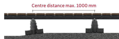
VARIO FIX with construction beams 80 x 60 mm
